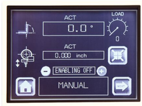
MANUAL Operator friendly single bend cycle. Displays actual bend position and current machine load.
