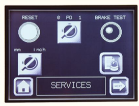
SERVICES Gateway to all machine services. Select multiple languages, monitor and adjust machine settings, view detailed alarm information, reset emergency stop, set pressure die ON/OFF and troubleshoot machine functions.
