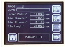
PROGRAM Select, enter and store program information, former radius, tube diameter, wall thickness and tube length.
